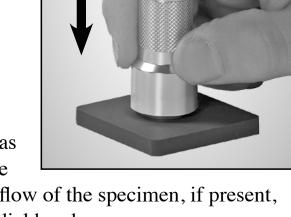
for several more seconds. Creep or cold-flow of the specimen, if present, will be evident by receding action of the dial hand.
